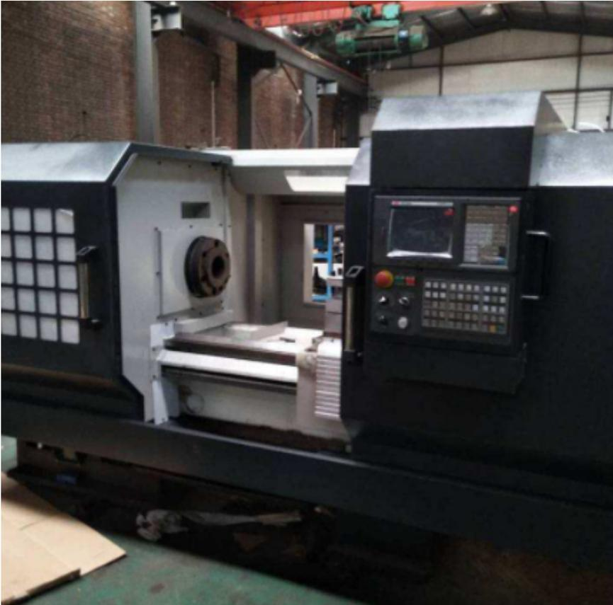
CNC machines have a logical approach to programming. Since the CNC control starts from zero at one point, the coordinate system must begin there. If the graph were a time line, the horizontal base line would start at January, while the vertical base line would start at a zero productivity level. This location is called the origin point. Various other names for the origin of a CNC machine are "work zero point," "part zero point," and "program origin."
