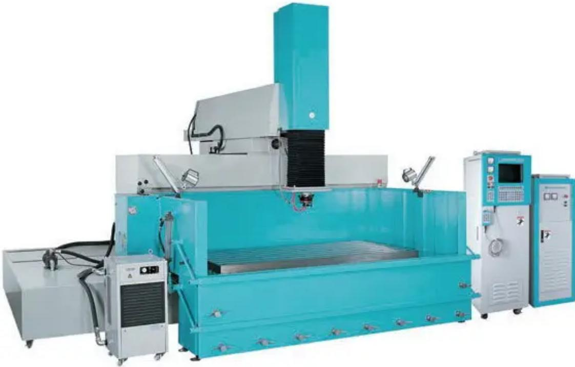
In an EDM process, the workpiece electrode is the electrode that changes shape to suit the purpose. This electrode is called the anode, and the tool is called the cathode. The two electrodes are separated by a dielectric fluid. A spark is produced in the process when the two electrodes make contact. The process results in a crater on the workpiece's surface.
