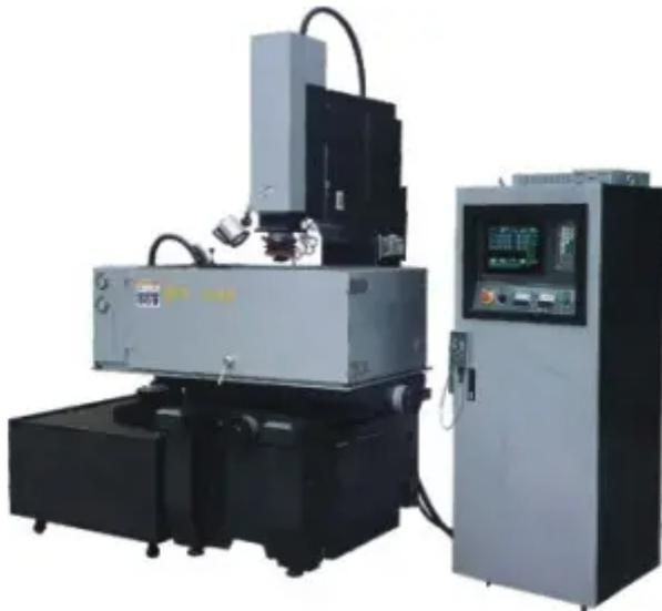
An EDM machine uses an electrode to make a hole in a workpiece. This electrode is typically a graphite wire but can also be copper. The electrode sinks into the workpiece and creates the three-dimensional shape, hole, or pattern. This process is highly accurate and precise. It is also relatively safe, as there is no need for special ventilation. When choosing a machine, make sure that it has a warranty period.
