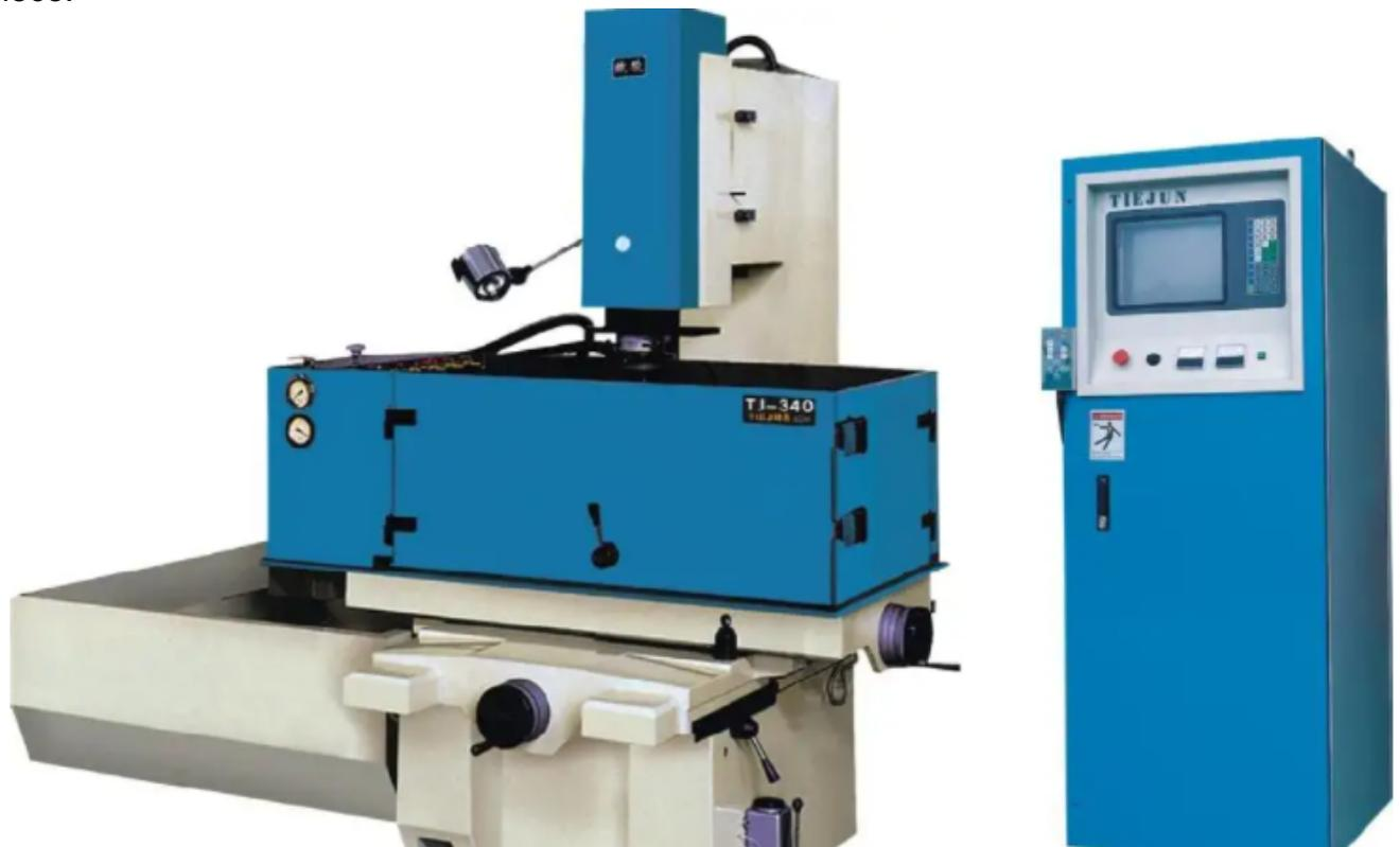
An EDM is used to size materials. The spark-driven tool electrode is immersed in the working fluid. The working fluid is charged into the discharge gap. The tool is fed through the gap by an automatic control system. The voltage generated by the electrical discharge breaks the working fluid and creates a spark. This action causes the sinker to break and form a hole. The resulting slit is the welded sinker.
