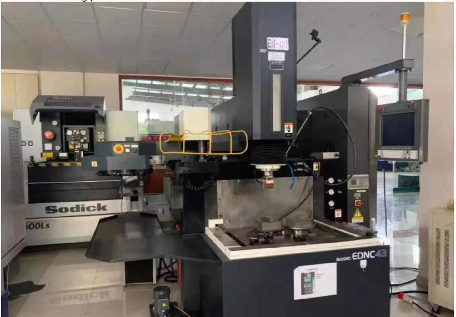
An EDM machine uses controlled electric sparks to cut and erode material. The workpiece never touches the electrode, which creates an insulating gap between the workpiece and the electrode. The amount of material removed by each spark is relatively small compared to the area impacted. The process also works well on plastics, as the materials are easily sanded. The electrical discharge machining machine for sinker can be used to manufacture plastics, molds, and a variety of other items.
