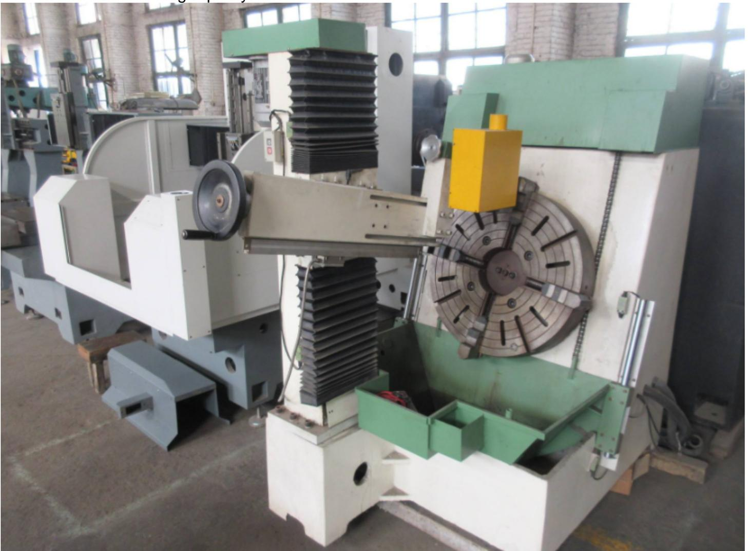
The most commonly used EDM machine for tire mould is the segmented tire mould EDM tool. It has a diameter of up to 1200 mm. The column tilts 15 degrees to facilitate iron pin discharge.
