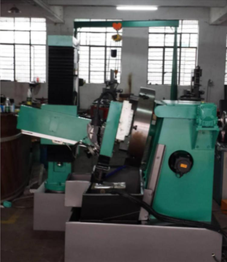
The EDM machine for tire mould has many benefits. It allows for better precision, as the EDM machine can be used to create complex shapes. Another advantage of the EDM machine for tire mold is that it can produce more complicated shapes. A conventional steel tire mold can be too deep, which means that electrodes have to be used for those deep areas. The newer equipment is also more accurate than manual methods.
