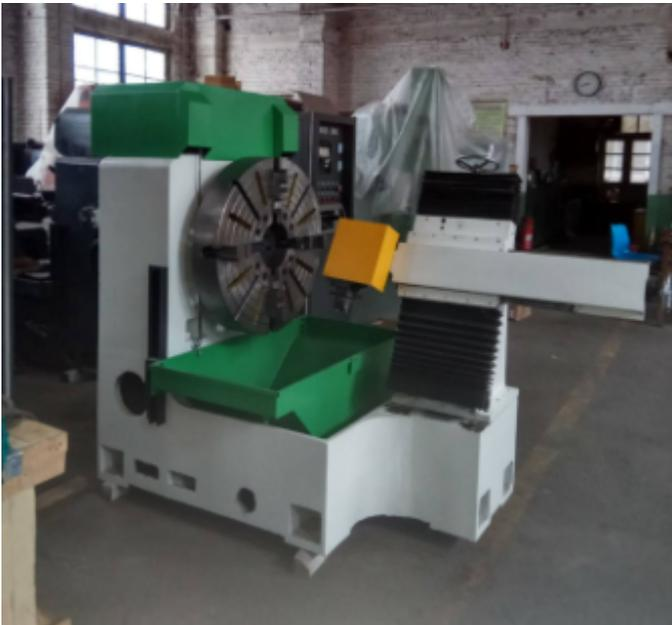
These machines are suitable for two-piece tire molding. You can easily change the parameters for each application. The F1050 is suitable for both types of applications.
