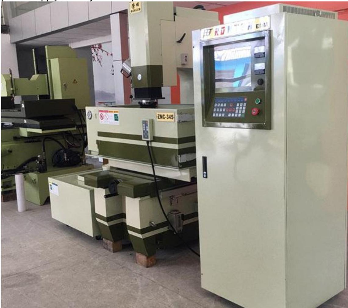
The wire electrode on an EDM machine breaks the dielectric fluid barrier, melting microscopic particles and eroding material. This process is repeated hundreds of thousands of times per second. The EDM machine controls the movement of the electrode and a dielectric fluid to cool the workpiece and electrode.
