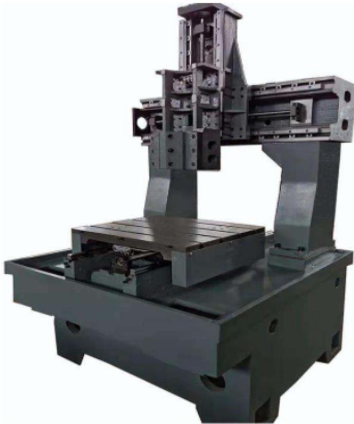
A milling machine uses a workpiece held on the table and moves it up and down the worktable, which controls the feed of the workpiece against the cutter.
